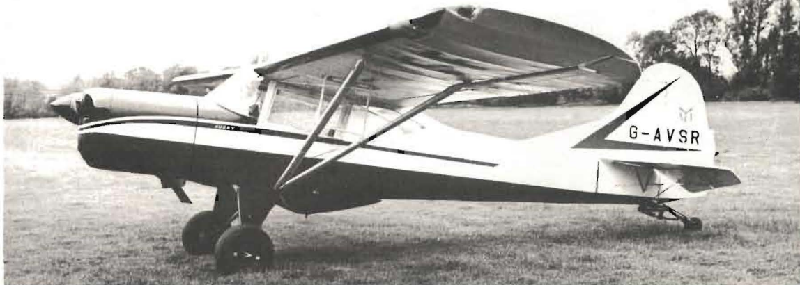
'VSR at Kingweston as she looks today. Clearly evident in this fine view is the belly-tank, flush landing and nav. lights, and the fitting of a spinner. Note also the owner's personal insignia on the aircraft's rudder. (ALY Aviation BWO2801)
