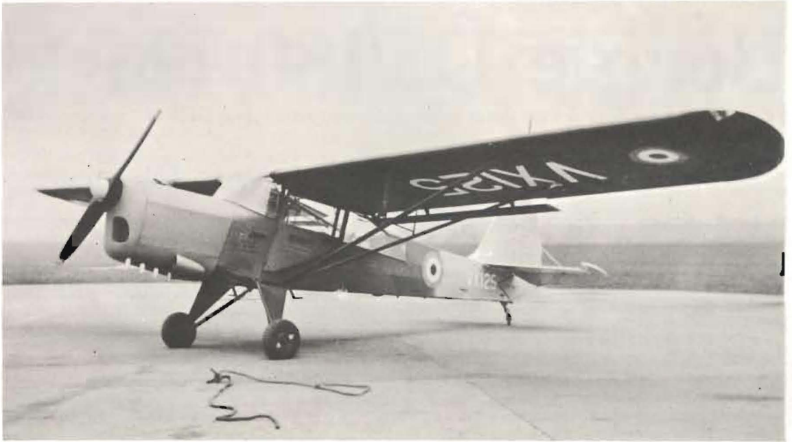
Above. AOP.6 VX125 was converted at Rearsby during 1950 as a test-bed for the new Blackburn Bombadier engine, as detailed on page 89. The unpainted tail surfaces show the amount of work needed in enlarging this area to offset the heavier engine. (John Lee)
